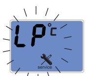
the code that identifies the cause is displayed, flashing, in place of the degrees centigrade, (for the "error codes" list see par. 4.6 installation and maintenance instruction manual).
