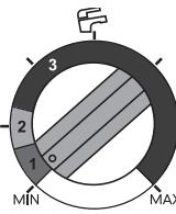
Via this knob it is possible to adjust the domestic hot water inlet temperature:
