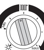
**Winter** (domestic hot water production and heating temperature adjustment). Positioning the knob in the field shown to the side, indicates that the boiler is in "Winter" mode, and adjusts the temperature of the heating circuit water. The adjustment is between min. 30°C and max 85°C.
