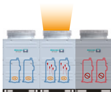
Outdoor Unit Backup
